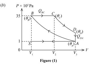
Figure (1) shows the standard *PV* cycle for a Diesel engine.  $\theta_A$ ,  $\theta_B$ ,  $\theta_C$  and  $\theta_D$  are the temperatures of the air mixture at the situations *A*, *B*, *C* and *D* respectively.
